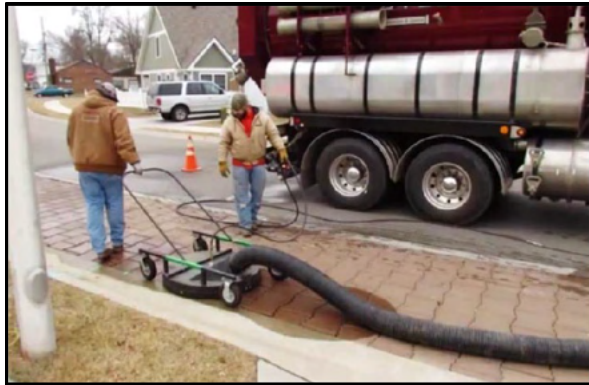
Combination Sewer Truck with 1,500 gallon water tank
