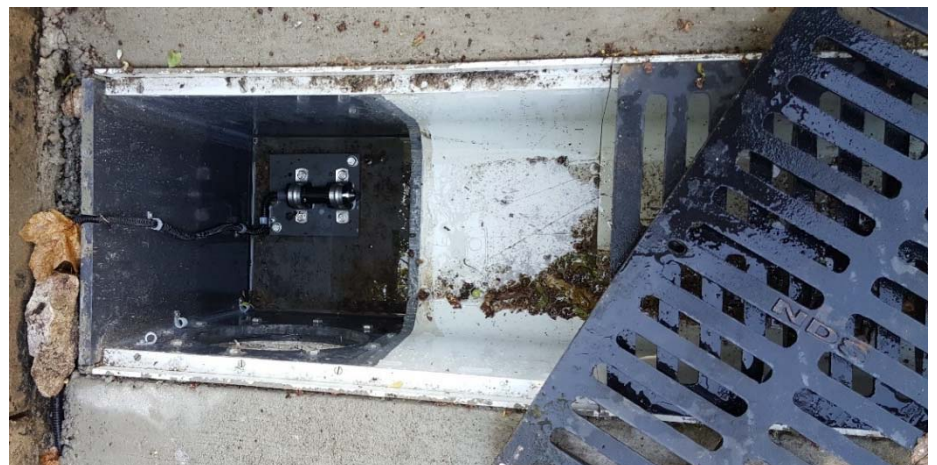
Pressure transducer mounted in bottom a sump box in a modified trench drain
