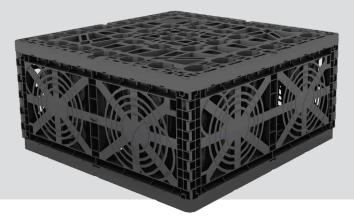
**PaveTank** offers the GRAF EcoBloc Maxx storage system for stormwater infiltration and retention solutions. This modular storage system has an HS-20 vehicle loading rating. Modules with baseplates can be stacked in multiple layers and mechanically connected to form almost any configuration – creating one of the lowest cost per cubic foot of underground storage available.
