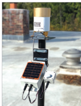
P4's INFIL-Tracker and Rain-mX transmit rainfall, stormwater captured, stormwater infiltrating, and when to clean the PaveDrain system.
