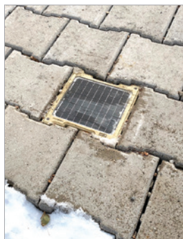
P4 INFIL-Tracker is battery powered, solar charged, and can be driven on.
