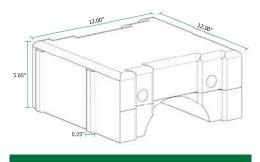
The PaveDrain block is 12" x 12" but also has two 0.25" Spacer Tabs on each side of the block. Please consider these when measuring.
